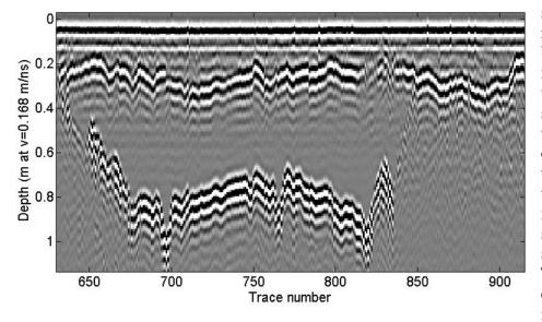
snow and ice in a riverine system behind a snow machine. We also used GPR to look at snow and ice thickness in specific cross-sections across the slough. We plan to extend these measurements to several of the main sections of the Tanana River that exhibit mid-winter ice degradation.
